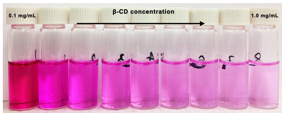
Figure 3.4 Phenolphthalein solutions with increasing \beta -CD concentration, where color faded from pink to colorless.
