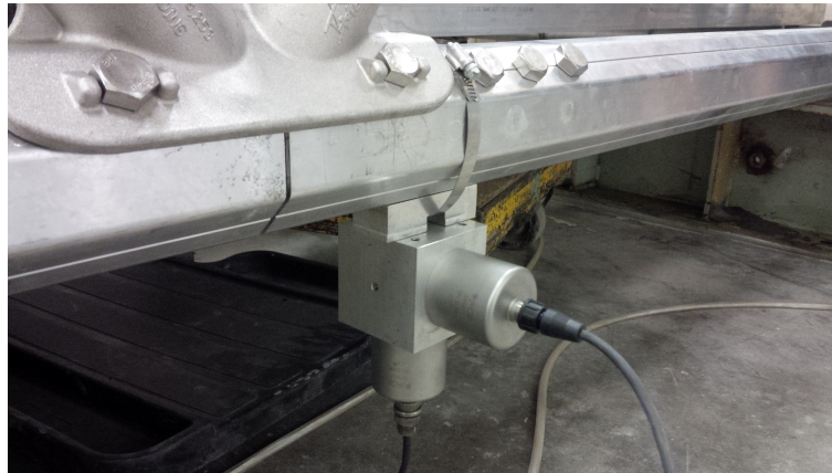
Figure 3.7: Accelerometer mounting system using hose clamp
