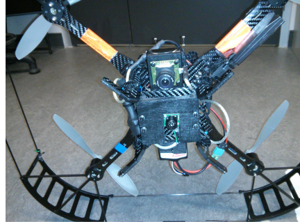
(b) The sonar and downward facing camera mounted on the bottom of the Pelican
