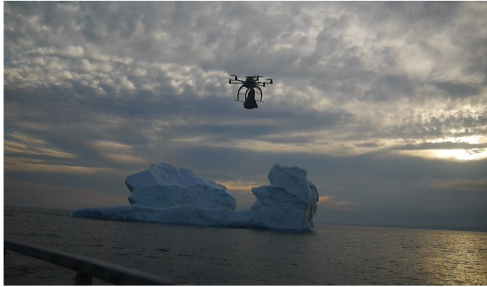
Figure 1.1: A hexacopter returns to a ship after dropping a GPS beacon on an iceberg.
