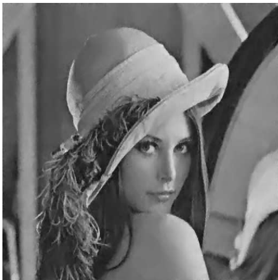
(c) Quadtree-based predictive fractal scheme collage error decomposition criterion RMSE=8.09, PSNR=29.97.
