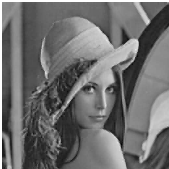
(c) LBG vector quantization RMSE=8.80, PSNR=29.24, C_R=22:1 . Execution time \approx 1534 secs.
