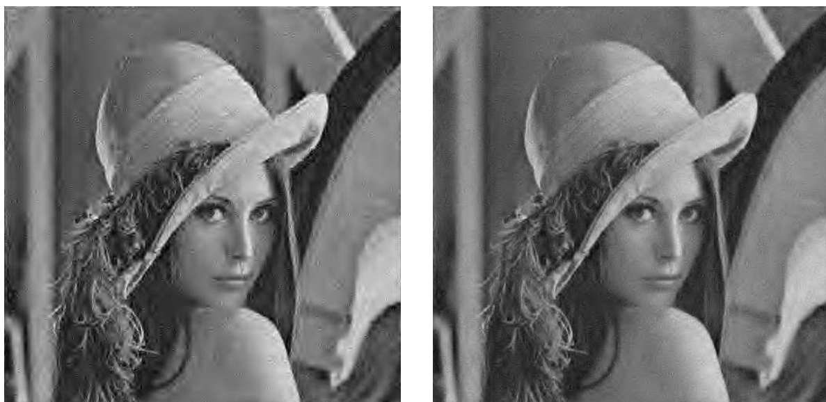
(a) Hard thresholding using: \lambda_{hard}^* = 80 RMSE=10.98, PSNR=27.31. Execution time \approx 8 secs.
