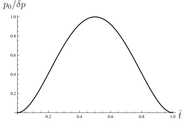
Figure 3.2: Normalized source p_0/\delta p for equation (3.23) as a function of the rescaled time \hat{t} = t/\delta t .
