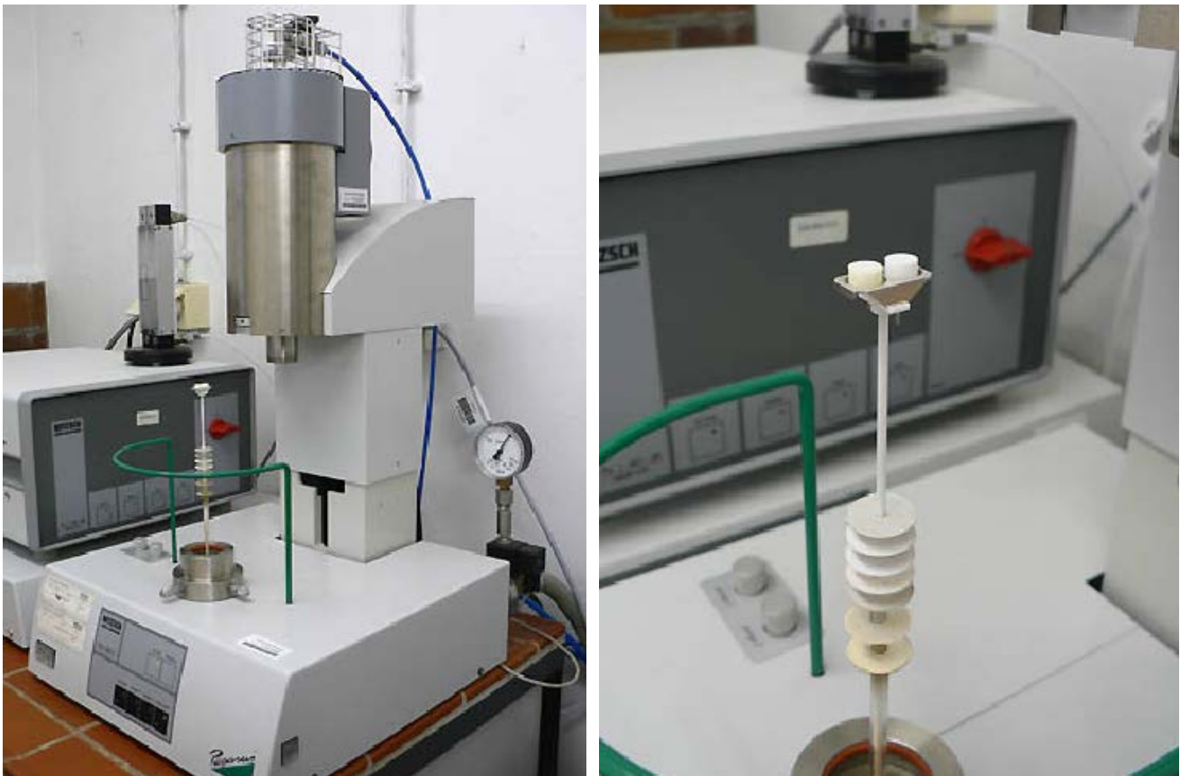
Figure 4-3 - (a) DSC Measuring Equipment with Controller and Gas Flow Monitor behind (b) Image of Sample Carrier with Alumina Crucibles
