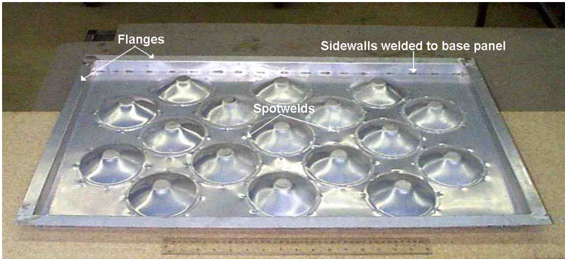
Figure 30: Assembled 1.0mm AA5754 inner panel with attached teacups and sidewalls with flanges. Teacup configuration #1 is shown.
