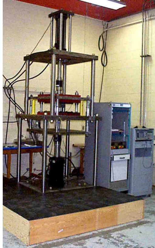
Figure 26: Hydraulic press at the University of Waterloo used to form the inner panel teacup supports.
