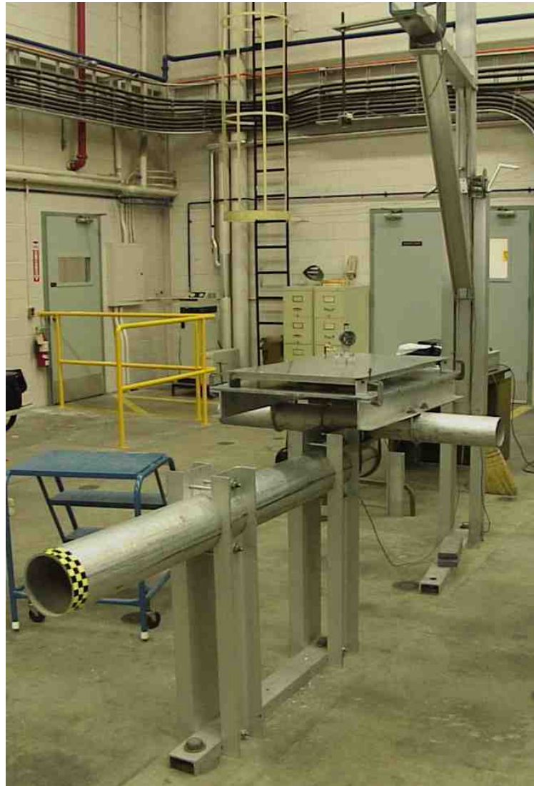
Figure 46: Dynamic denting test setup.
