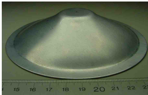
Figure 28: Formed and trimmed AA5754 inner teacup support.
