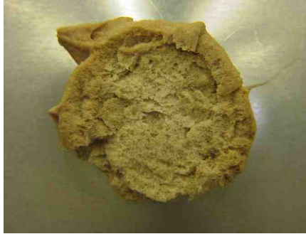
Figure 41: Cured automotive mastic on top of a teacup after removal of the outer panel exhibiting good mastic coverage and adherence.
