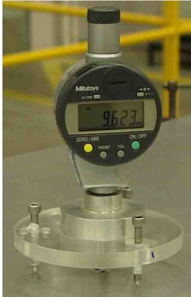
Figure 51: Close-up of dial gauge mounted on tripod platform. Three adjustable screws allow for leveling of the platform above the dent site to assure normal measurements. The screws are 38mm from the centre of tripod.
