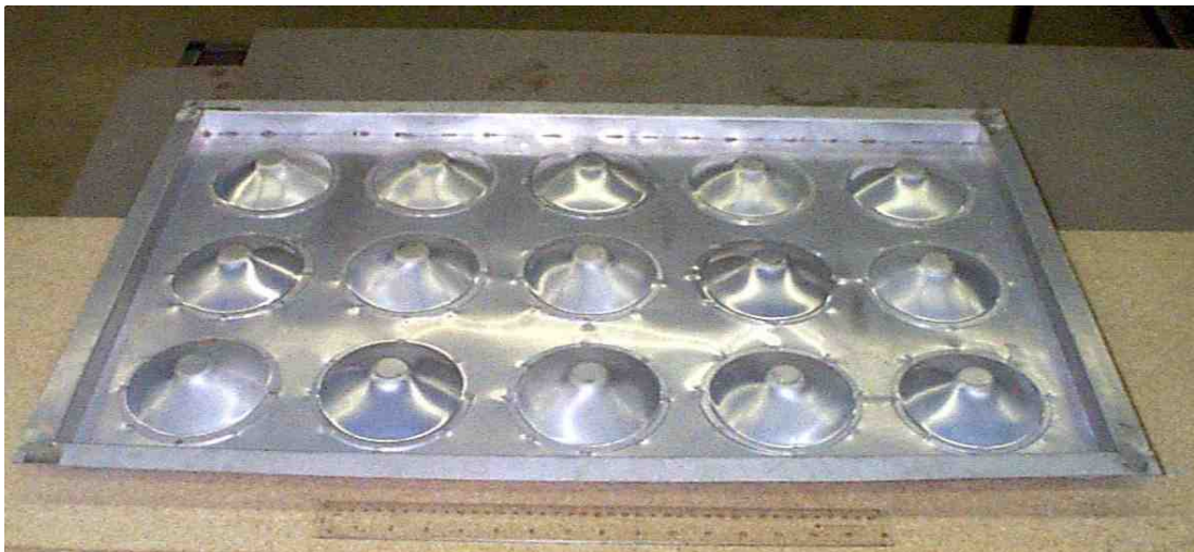
Figure 31: Assembled 1.0mm AA5754 inner panel with attached teacups in configuration #2.
