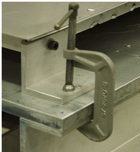
Figure 36: Close-up of inner panel mounting bracket for attachment to dent testing rig.
