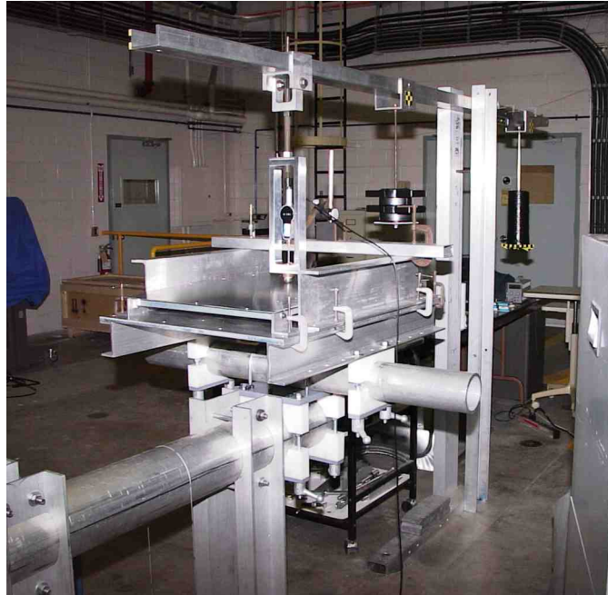
Figure 55: Test rig configured for static dent testing.
