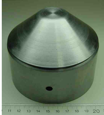
Figure 27: Final modified 101.6mm diameter, conical flat-topped punch used to form the teacups.
