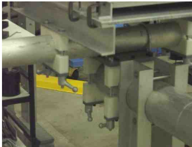
Figure 48: Close-up showing the rotational clamps on the denting test rig. The clamps can be unlocked allowing the cylinders to rotate freely in the supports.
