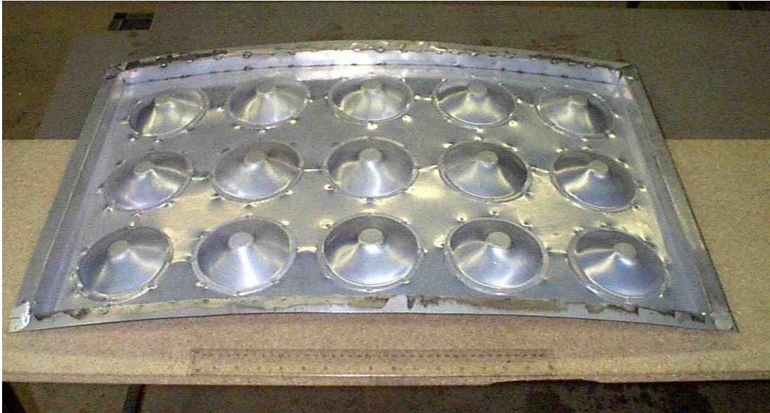
Figure 32: Assembled 1.0mm AA5754 medium curvature inner panel with attached teacups in configuration #2.
