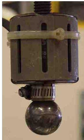
Figure 49: Close-up showing electromagnetic indenter release mechanism at end of the dynamic denting alignment arm. The 25.4mm spherical steel indenter is held by an alignment nut at the end of the threaded rod.
