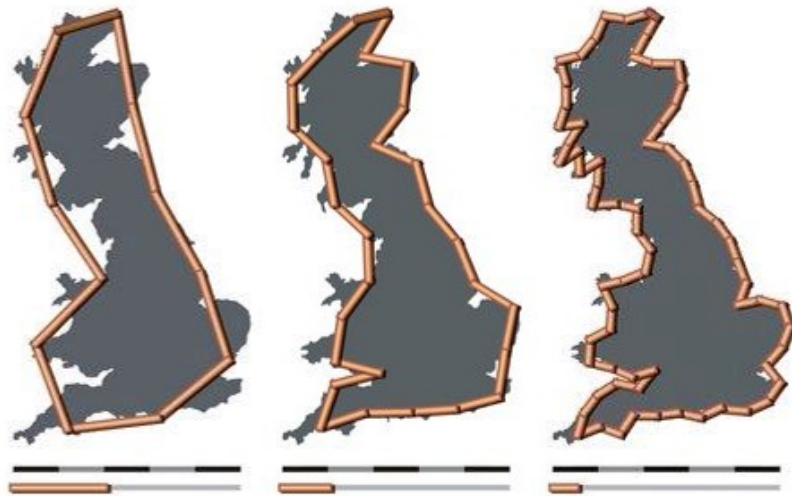
Figure (2-1): Illustration of the coastline paradox. From left to right, the coastline of Britain is measured by 200 km, 100 km, and 50 km rods, resulting in 2350 km, 2775 km and 3425 km length of coastline respectively (Van de Sande, 2004).
