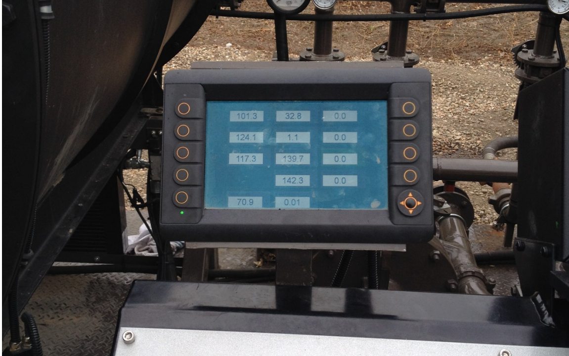
FIGURE 3.4: As-mounted configuration of the CR1081 screen with sample UI.
