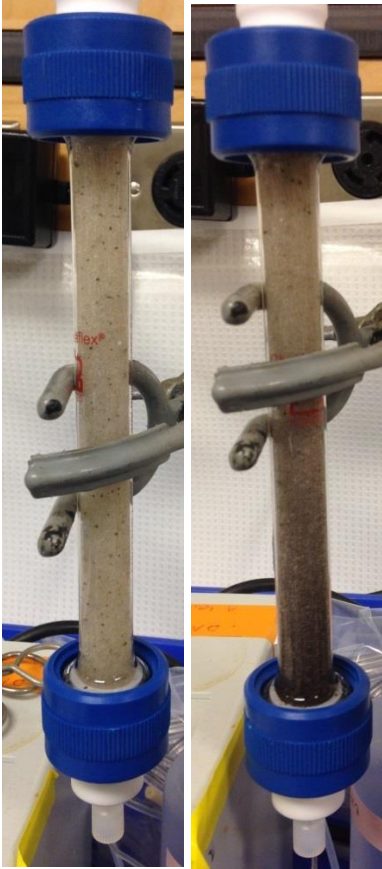
Figure A.12. Before and after (0 and 20 pore volumes) photographs from CSA-340 in 5.1 mM IS CaCO 3 column test showing the retention of 5 PV of nanoparticle input.
