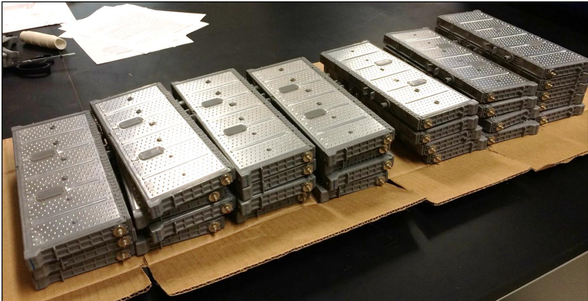
Figure 52: Disassembled Battery modules
