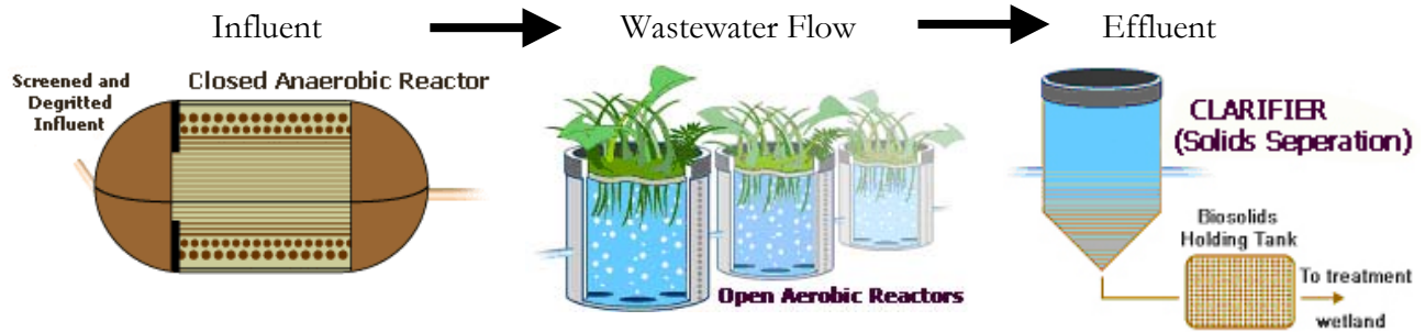
Figure 2-3. Illustration of Greenhouse Treatment Technology. Source: Living Machines Inc. (2002)
