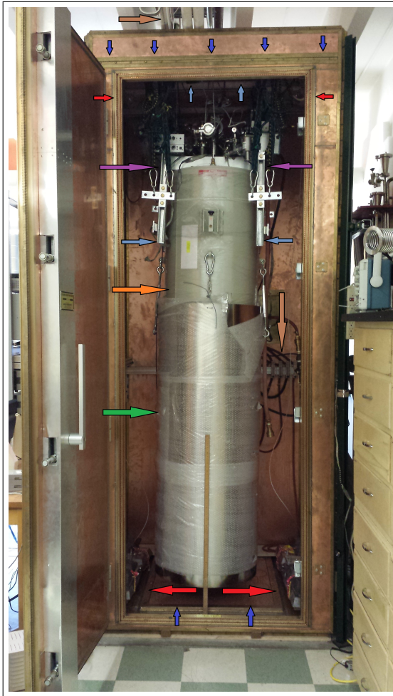
Figure 4.7: The dilution refrigerator sitting inside of the dewar during a cooldown. The arrow colors are as follows: Dark blue: RFI/EMI shielded room with removable floor. Green: Mu-metal shield. Orange: liquid Helium dewar. Brown: Gas manifold in the back of the room connecting the dewar to a system of pipes at the back of the room, which come over the roof and lead to the Helium recovery system. Red: Lead counterweights which wrap around pulleys located at the top of the room. Purple: Hard to see bungee cords holding the 650 lb load up on a unistrut frame, there are 2 sets of bungees in the front and 2 sets at the back. Light blue: The unistrut frame holding everything up, which is connected to a unistrut reinforced ceiling through the bungee cords when in operating mode, or through the counterweights when not operating.
