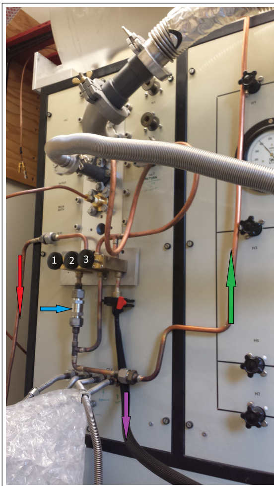
Figure 4.5: The manifold installed on the gas handling system. The purple arrow leads to the return side of the fridge. By closing valve 3, and opening valve 2, the mix can be sent to backup storage tanks on the top of the gas handling system, (indicated by the green arrow). Here, they can be circulated through external cold traps without running through the dilution unit. With valve 3 open, 2 closed, and 1 open, the fridge is in normal operation mode but with an extra safety, namely the red arrow which leads to the back of the rotary pump of the gas handling system. In the event of the pressure at the back of the rotary pump exceeding 5 psi, a pressure relief valve indicated by the blue arrow opens which will vent the mix to the backup storage tanks on the top of the gas handling system.
