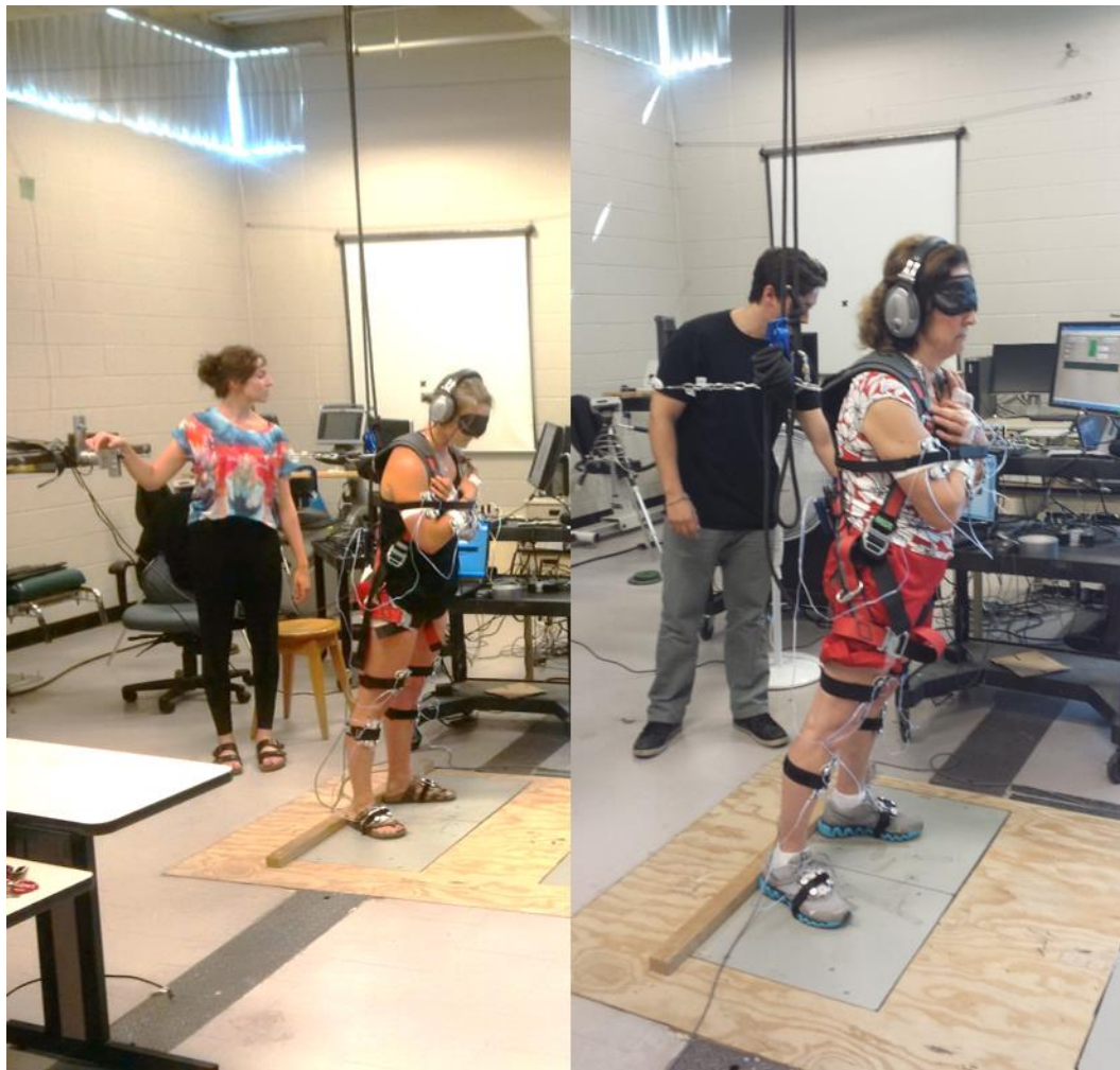
Figure 10. Lean and release cable set-up for both younger and older adults. Participants were blindfolded and instructed to lean forward such that their body weight was supported by the cable from neutral stance. Perturbation onset time was calculated by a mounted load cell attached
