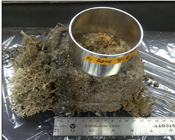
Figure 3-6. Peat core extraction for HYPROP and KSAT experiments. Metal core ring (250 ml) for HYPROP and KSAT used to extract a sub-core from the larger peat core for determining horizontal conductivity.
