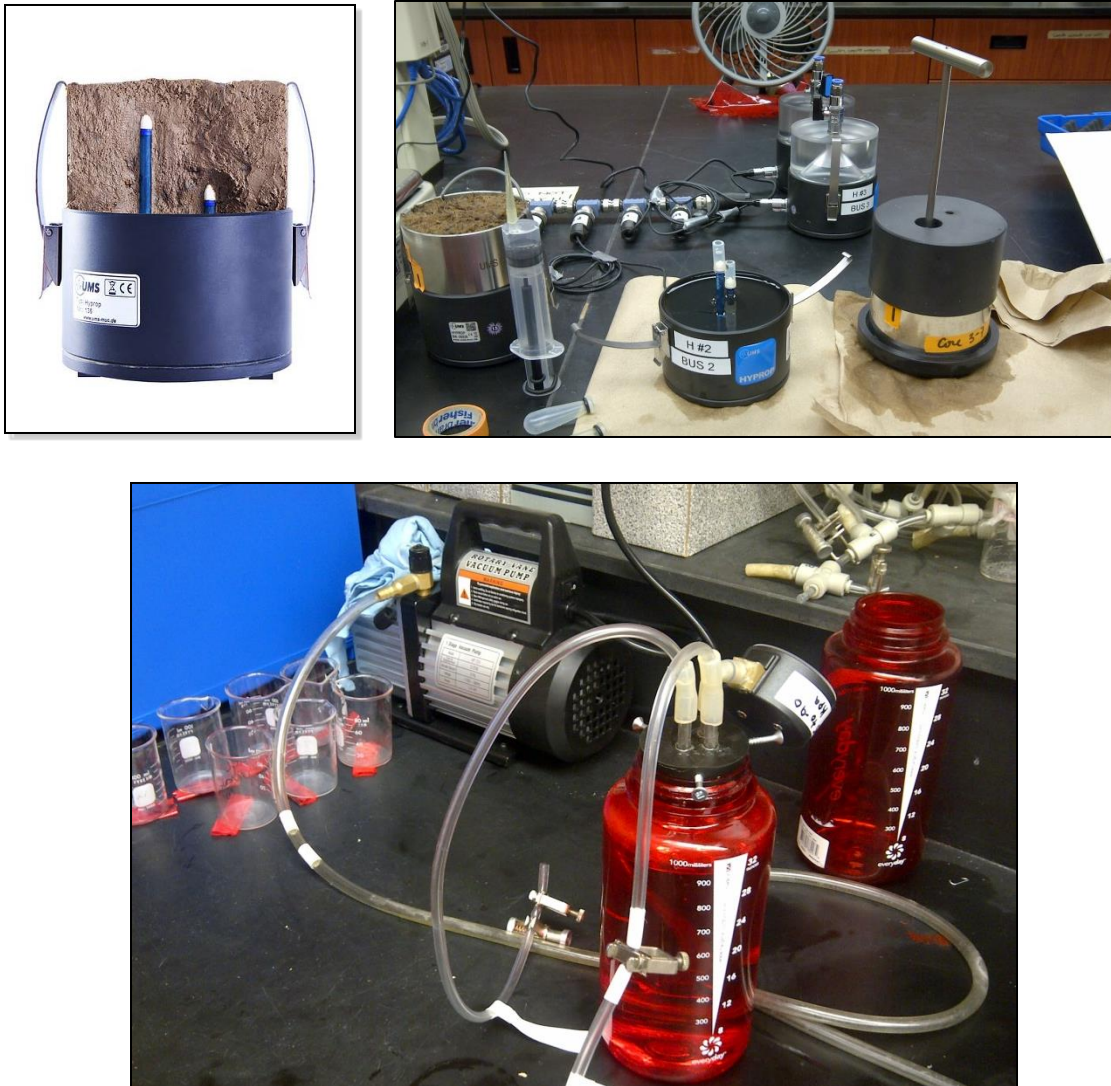
Figure 3-1. Top: HYPROP core preparation. Top left: Visual of the two tensiometers within the soil core and HYPROP base, taken from http://www.ums-muc.de/en/products/soil_laboratory/hyprop.html . Top right: Preparation of the HYPROP bases and soil cores for the HYPROP evaporation experiment. Bottom: HYPROP base degassing preparation. Because of the sensitive nature of the HYPROP base pressure sensor, a secondary ‘buffer bottle’ (at right, without lid) was also attached to the main chamber bottle seen in the front with the pressure gauge on top. See also Figure 3-2.
